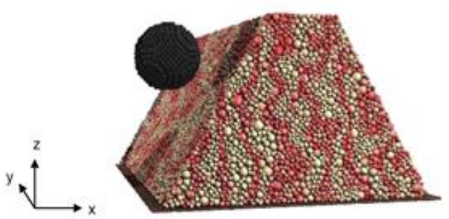
Figure 31 DEM model of embankment and block, both made of “glued” spheres (Plassiard and Donzé, 2010)
